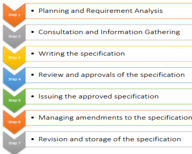
Figure 2.1: Typical Specification Process Flow4
